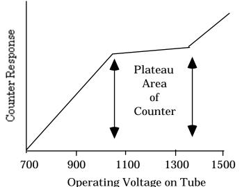
Fig. 2: Response of G-M tube as a function of applied voltage.
