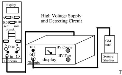
Fig. 1: Counter setup for radioactivity experiments
