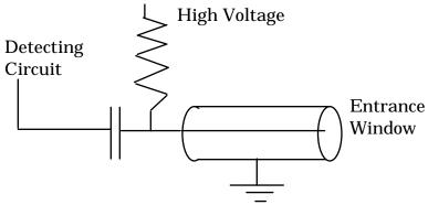
Fig. 1: Schematic of a Geiger-Mueller Tube.
