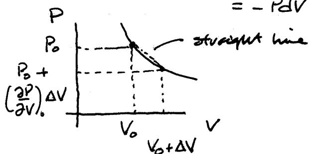
$$U = P_0 \Delta V + \frac{1}{2} \left( \frac{\partial P}{\partial V} \right)_0 (\Delta V)^2 \quad \text{straight line app.}$$
