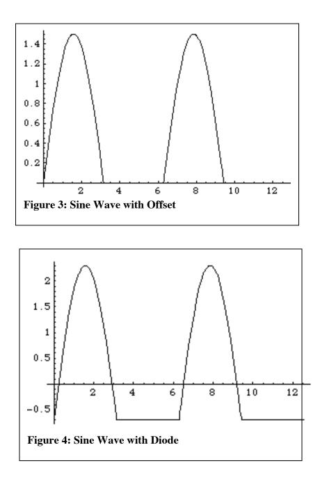
**Experiment**: Vary the level of the sine signal and the offset so that you see an output like Figure 4. Then set the level and the offset so that the output resembles Fig. 2.
