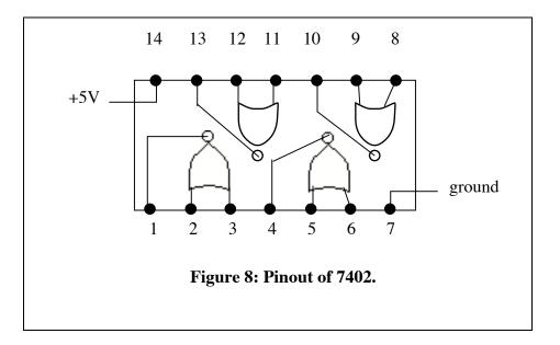
**Experiment**: Verify the NOR truth table for one or two of the logic gates of a 74LS02: [This chip also needs a +5 volt supply at pin 14 and a ground at pin 7.]
