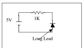
Figure 9: PIN Diode Circuit.
