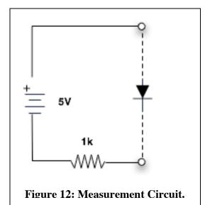
Reverse the diode to attempt to find the effect of light on the diode current in the forward-biased condition.
