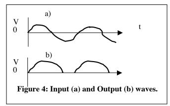
The basic half-wave rectifier with resistive load looks like the circuit above. The Input and Output waveforms are shown on the right.
