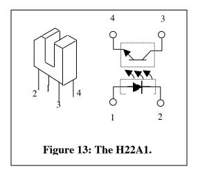
Build the circuit in Figure 14 using an H22A1 from Harris Semiconductor or an alternate device from Fairchild. The pinout for the latter is available on a datasheet pasted to a cabinet in the lab.
