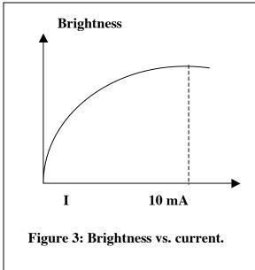
function of current as you increase the supply voltage. You should find that a current between 5 and 10 mA gives a normal glow.
