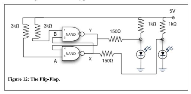
Build the flip-flop and test it.
