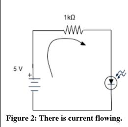
In Figure 1 the diode is biased in the backward direction or "reverse biased" and there is no current flowing through it whereas in Figure 2 the diode is "forward biased" and there is current flowing. Note that the longer lead of the diode indicates + side.
