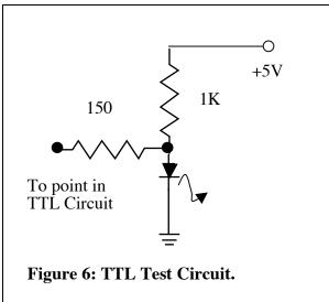
The answer to the question on Figure 5 is: "about 3 mA". We use the circuit shown in Figure 6 to determine whether a point in a TTL circuit is logically high or logically low. If it is high then this point will not cause much voltage drop on the 1K resistor and the LED will glow. If the point is low then it will sink current, causing a voltage drop on the 1K resistor, and the LED will not glow.
