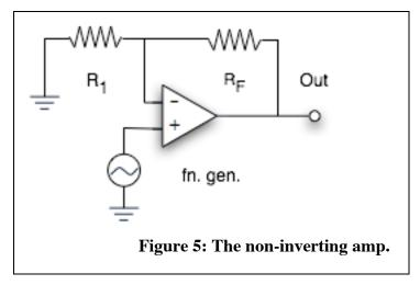
(a) \*Show mathematically that you expect the gain to be given by  $1 + R_f/R_1$ . Measure the gain to verify this using resistor values in the range 3K to 200K.
