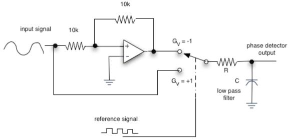
The figure below shows a basic phase detector.
