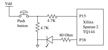
Figure 5. Pushbutton and LED detail
