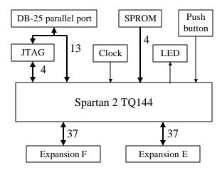
D2XL FPGA circuit block diagram
