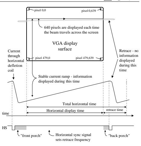
back porch intervals (porch intervals are the pre- and post-sync pulse times during which information cannot be displayed) are based on observations taken from VGA displays.
