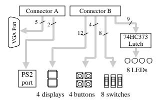
Figure 1. DIO1 schematic
