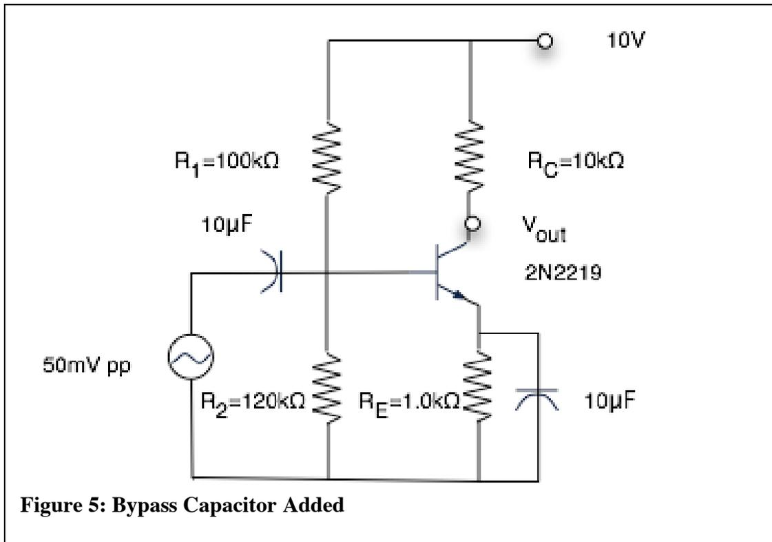
**Figure 5: Bypass Capacitor Added**
