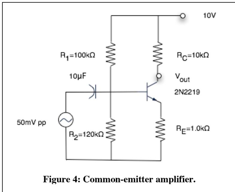
**Figure 4: Common-emitter amplifier.**
