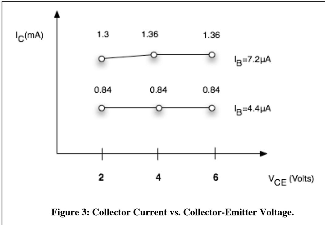
Figure 3: Collector Current vs. Collector-Emitter Voltage.
