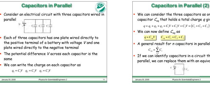
We can consider the three capacitors as one equivalent capacitor  $C_{eq}$  that holds a total charge q given by  $q = q_1 + q_2 + q_3 = C_1 V + C_2 V + C_3 V = (C_1 + C_2 + C_3) V$ • A general result for *n* capacitors in parallel is If we can identify capacitors in a circuit that are wired in parallel, we can replace them with an equivalent capacitance
