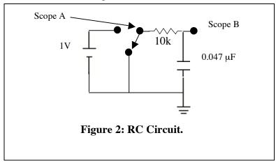
In lecture you will learn that this circuit can be described by a differential equation for q(t), the charge on the capacitor as a function of time. If you have time, you may wish to write down the equation and show that a solution for the voltage on the capacitor,  $V_C = q(t)/C$ , consistent with no initial charge on the capacitor, is:
