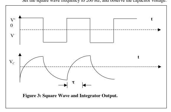
Use the 'scope to measure the time required to rise to a value of  $(V_+ - V_-)(1-e^{-1})$ . Accuracy in this measurement is improved if the pattern nearly fills the screen. This rise time must be equal to  $\tau$ . Compare with the calculated value of  $\tau$ .
