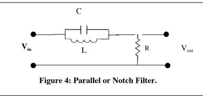
\* Explain why this is a notch filter. What is the frequency of the notch? Use L = 27 mH, C = 0.047  $\mu$ F and R = 150  $\Omega$ . Measure the depth of the notch by comparing the response at the bottom of the notch with the response at low or high frequency. Why doesn't the response go to zero at the bottom of the notch?
