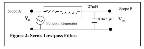
Notice that there is no discrete resistor. The resistor in this circuit is the resistance of the inductor plus any resistance contributed by the Function Generator. Normally the Function Generator has an output impedance of 50  $\Omega$ . Verify that this is the case. Use an ohmmeter to measure the resistance of the inductor, add the value contributed by the Function Generator and use this sum in your calculations below.
