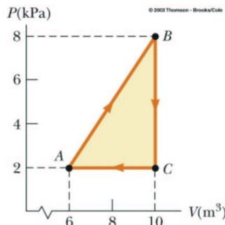
A gas is taken through the cyclic process described by the figure above. How much work was done by the gas during the cycle ABCA? (in J)
