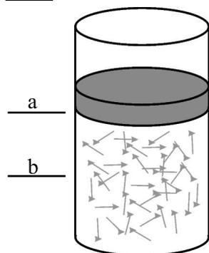
A massive piston traps a fixed amount of helium gas as shown. After being brought to point (a) the system equilibrates to room temperature. The gas is then cooled ISOBARICALLY compressing the gas to half of its original volume (b).
