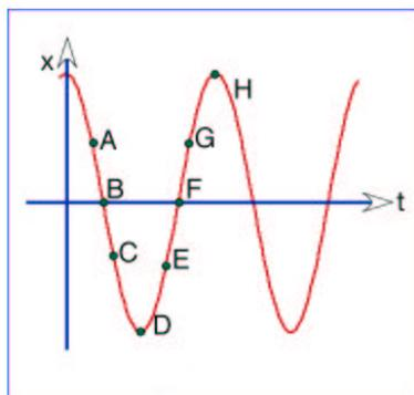
The curve represents an object in simple harmonic motion. Match the points on the curve to the velocity and acceleration of the object.
