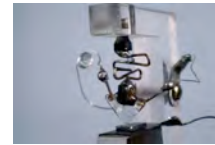
Replica of first transistor in 1947
