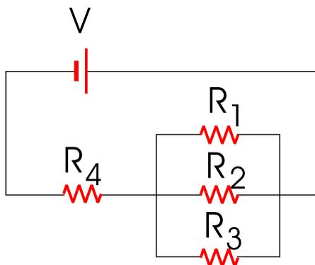
Assume that  $V = 30.5 \text{ V}$ ,  $R_1 = 15.7 \Omega$ ,  $R_2 = 8.19 \Omega$ ,  $R_3 = 4.58 \Omega$  and  $R_4 = 18.8 \Omega$ .
