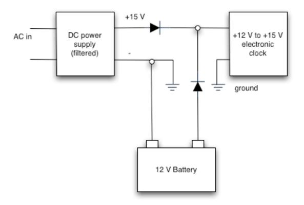
Make a simple modification to the circuit so that the battery is charged by the dc supply (when power is on, of course) at a current of 10 mA (such a circuit is necessary to maintain the battery's charge).
