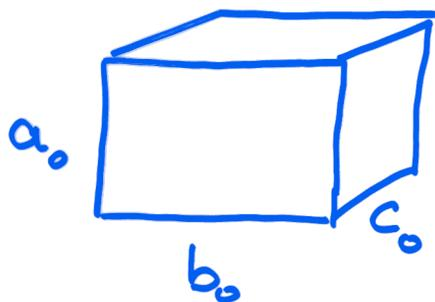
$$V_0 = a_0 b_0 c_0$$
