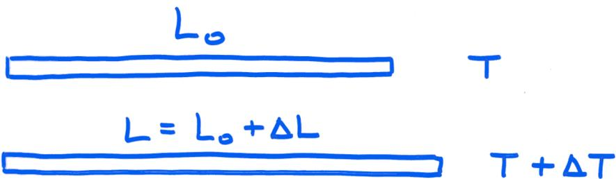
$$\left. \begin{array}{l} \Delta L \sim \Delta T \\ \Delta L \sim L_0 \end{array} \right\} \Rightarrow \begin{array}{l} \Delta L = \alpha L_0 \Delta T \\ L = L_0 (1 + \alpha \Delta T) \end{array}$$
