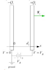
Voltage constant at  $V_{\rm B}$ Charge changes to  $Q_1$
