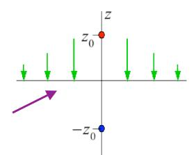
E field on conductor's surface = E field of dipole on the midplane
