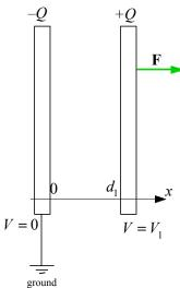
Charge constant at Q Voltage changes to  $V_1$
