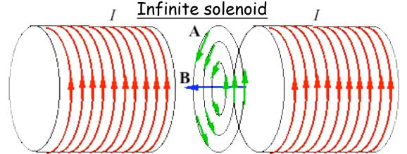
Cut-away drawing showing the axial magnetic field B (uniform), and growing circular vector potential A.
