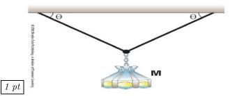
A lamp is hung as shown where the angle of the support wires is  $\theta = 45$  degrees. If the maximum tension either wire can handle is 45 lbs, what is the maximum weight of a lamp that can be supported? (in lbs)
