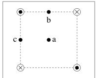
Two currents go into the page, and two are pointing out of the page. Point **a** is at the center of the square, and points **b** and **c** are in the middle of two of the sides.
