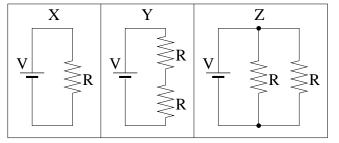
5 pt Select the circuit with the smallest voltage drop across a single resistor.
