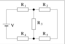
6 pt What is the equivalent resistance of the circuit? (*in* ohm)
