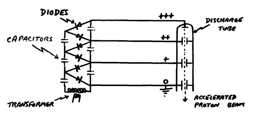
I'VE ILLUSTRATED A 3-STAGE STACK. THE DISCHARGE TUBE WOULD BE CHARGED UP TO 600 KV, THE FIRST ELECTRODE WOULD BE AT 400 KV, THE NEXT AT 200 KV AND THE BOTTOM ONE AT GROUND. A PROTON WOULD GAIN 200 KeV AT EACH STAGE.
