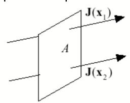
Current is charge through A per unit time
