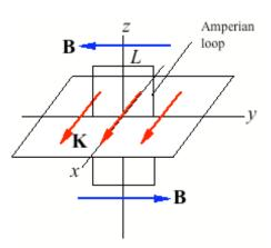
Infinite current slab
