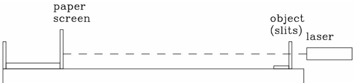
Figure 2: Diagram of the optical bench (side view).
