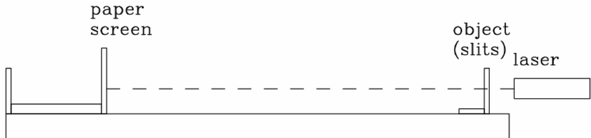
Figure 2: Diagram of the optical bench (side view).
