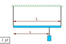
Two wires support a beam of length L=16 m as shown in the figure above. A box hangs from a wire which is connected a distance of 12 m from the left edge of the beam. The tension in the left support wire is 700 N and the tension in the right support wire is 900 N. What is the mass of the beam? (in kg)
