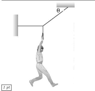
Consider the cat burglar of mass 59 kg in the figure, where the angle  $\theta$ =33 degrees. What is the tension in the horizontal section of the cable?
