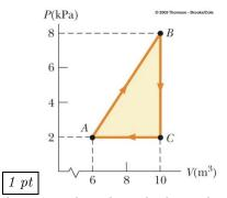
A gas is taken through the cyclic process described by the figure above. How much work (in J) was done by the gas during the expansion from A to B.
