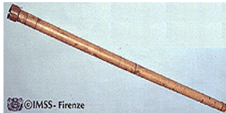
Wood, paper; length: 1360mm, lens diameter 26mm http://galileo.imss.firenze.it
