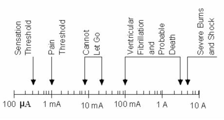
Figure 3 Effects of current (60 Hz)
