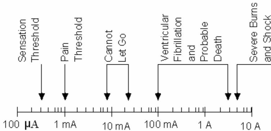
Figure 3 Effects of current (60 Hz)
