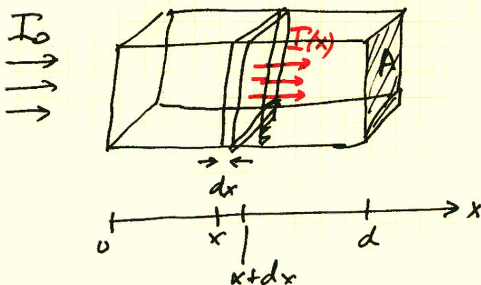
$$I(x) = \# \text{ photons/m}^2/\text{sec} \text{ at } x$$
