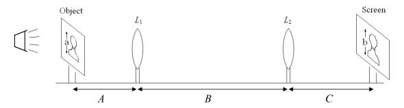
The image produced by the first lens  $L_1$  appears at position  $s_1^{'}$  and is given by
