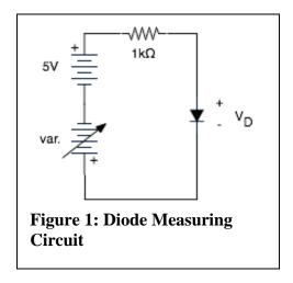
characteristic to show the rapid rise in forward current when the forward voltage approaches 0.7 volts. It should look something like the curve in Figure 2.
