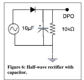
The capacitor is electrolytic. You must obey the polarity markings when you connect this capacitor in the circuit.
