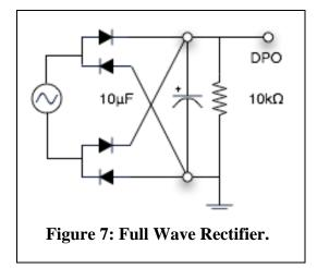
Build the circuit above. Use a 10 V peak to peak, 60-Hz signal.
