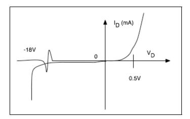
Figure 2: Diode Characteristic Curve
