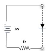
**Figure 12: Measurement Circuit**
