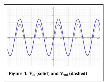
The basic half-wave rectifier with resistive load looks like the circuit in Figure 3. The Input and Output waveforms are shown Figure 4.
