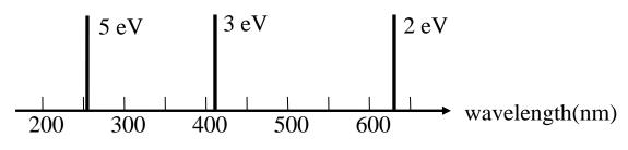
QM1-71. The spectrum of "Perkonium" has 3 emission lines
