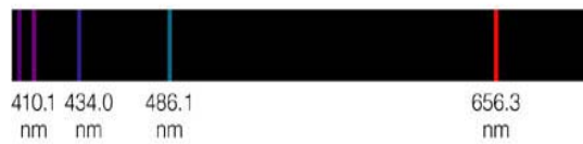
Emission spectrum of hydrogen
