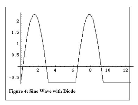
**Experiment**: Vary the level of the sine signal and the offset so that you see an output like Figure 4. Then set the level and the offset so that the output resembles Fig. 2.
