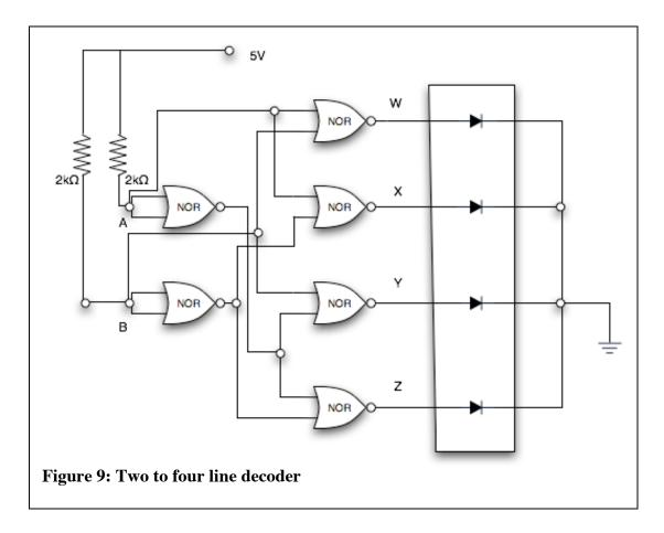
Calculation: Complete the truth table for the four outputs w, x, y, and z, given the four possible inputs from lines A and B.
