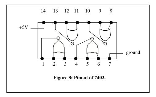
Experiment: Verify the NOR truth table for one or two of the logic gates of a 74LS02: [This chip also needs a +5 volt supply at pin 14 and a ground at pin 7.]
