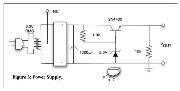
The rectangular box refers to the full-wave rectifier WL02F. and "NC" means no connections to the center tap on the transformer The output should be about 5 volts.
