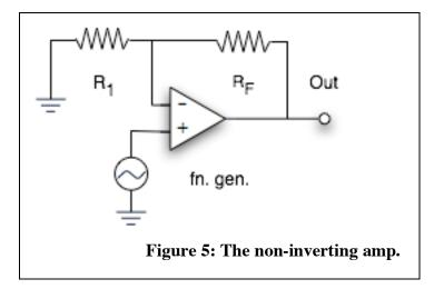
(a) \*Show mathematically that you expect the gain to be given by  $1+R_f/R_1$ . Measure the gain to verify this using resistor values in the range 3K to 200K. Paste a copy of an example DPO screen in your notebook.
