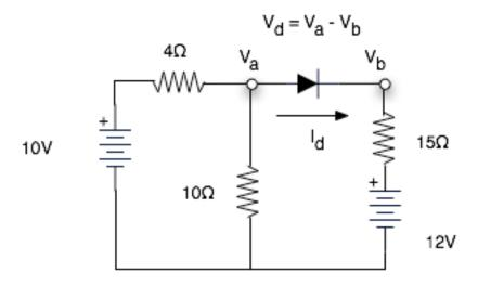
Find the voltage  $V_{\text{d}}$  and current  $I_{\text{d}}$  for the diode in the circuit above. Assume a perfect diode.
