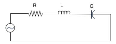
For the circuit shown, draw the phasor diagram including all voltages. Assume  $\omega$  = 100 rad/s, L = 1H, C = 50  $\mu$ F, R = 100 $\Omega$  and source voltage V = 200 V sin $\omega$ t.
