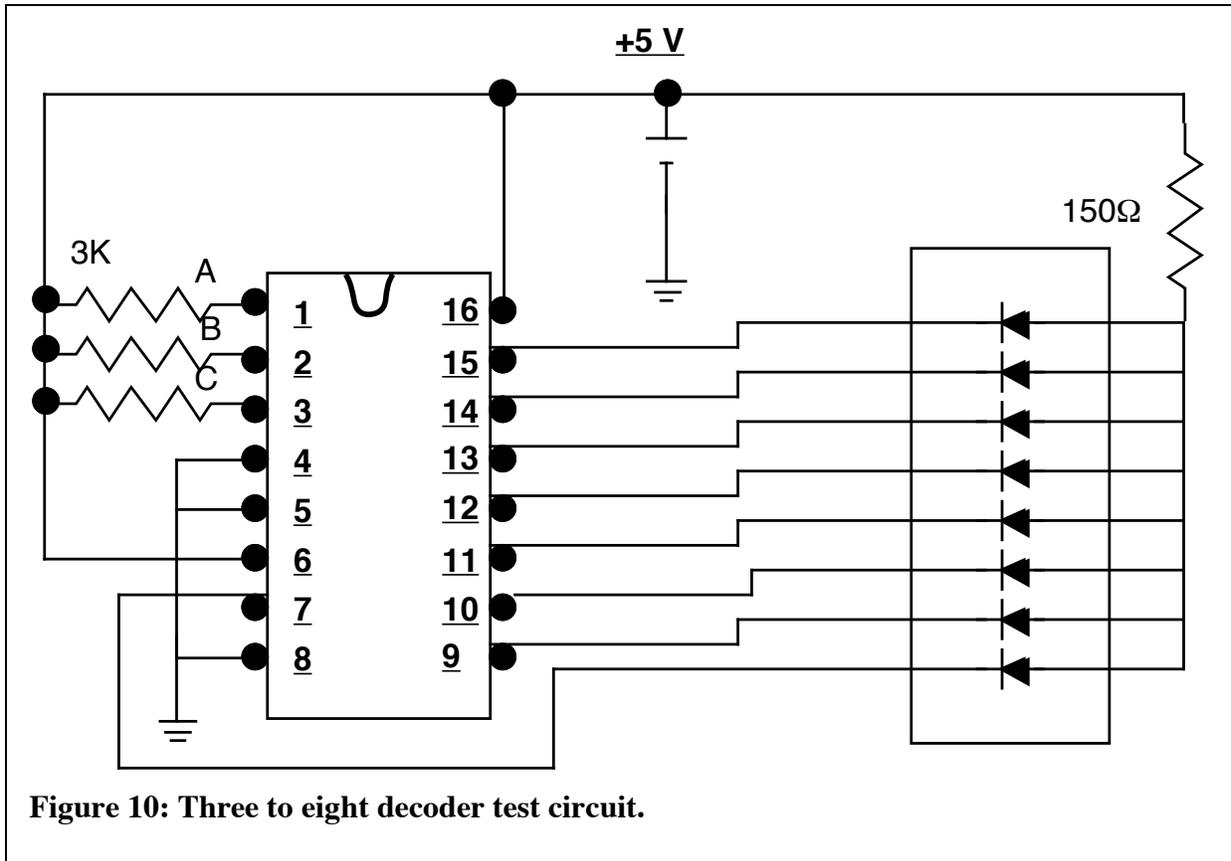
Figure 10: Three to eight decoder test circuit.
