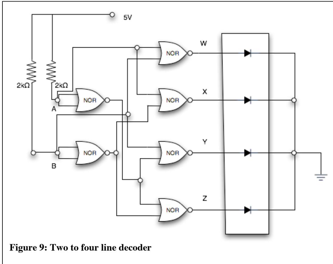
**Calculation:** Complete the truth table for the four outputs w, x, y, and z, given the four possible inputs from lines A and B.
