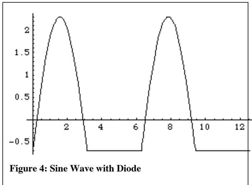
Experiment: Vary the level of the sine signal and the offset so that you see an output like Figure 4. Then set the level and the offset so that the output resembles Fig. 2.
