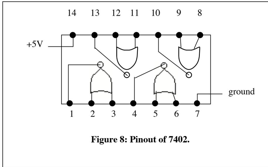
**Experiment:** Verify the NOR truth table for one or two of the logic gates of a 74LS02:
