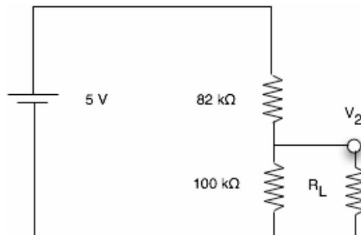
**Figure 3: Voltage Divider.**
