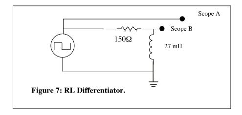
Calculate time constant  $\tau = L/R$ . Remember to include the resistance intrinsic to the inductor in R as well as a  $50\Omega$  resistance contributed by the pulser. Measure the time constant on the DPO and compare with the calculated value.
