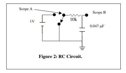
In lecture you learned that this circuit can be described by a differential equation for q(t), the charge on the capacitor as a function of time. It was shown that a solution for the voltage on the capacitor,  $V_C = q(t)/C$ , consistent with no initial charge on the capacitor, is:
