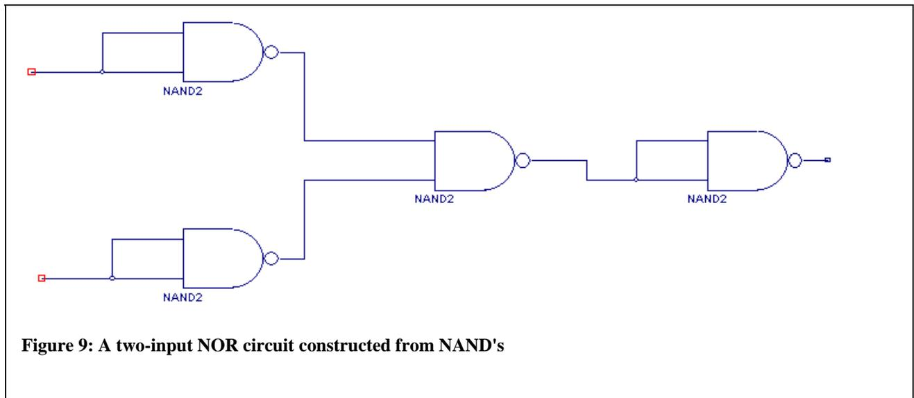
Figure 9: A two-input NOR circuit constructed from NAND's
