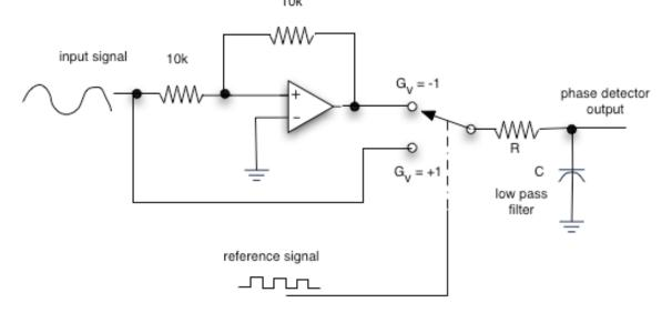
An analog signal passes through a linear amplifier whose gain is reversed by a square-wave "reference" signal controlling an FET switch. The output signal passes through a low-pass filter, RC.
