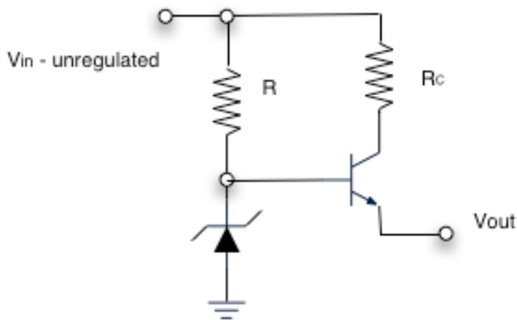
The resistor  $R_C$  protects the transistor by limiting maximum output current.
