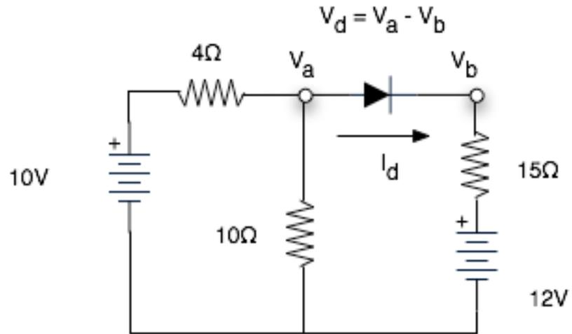
Find the voltage  $V_d$  and current  $I_d$  for the diode in the circuit above. Assume a perfect diode.
