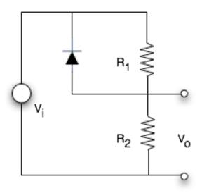
Plot  $V_0$  vs.  $V_i$  for the circuit above. Assume that the diode is perfect, the input voltage varies in the range -10V <  $V_i$  < 10V and  $R_1$  = 10  $R_2$ .
