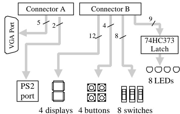
Figure 1. DIO1 schematic
