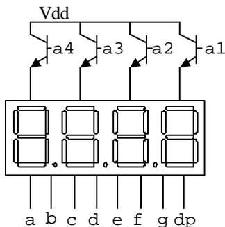
**Cathodes** -- connected to CPLD pins via 100 Ω resistor
