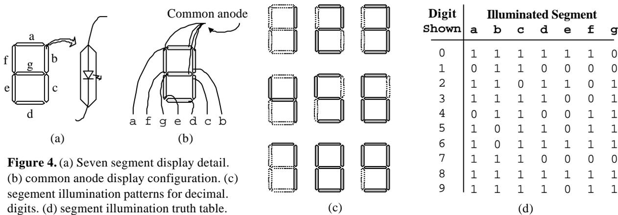
**Figure 4.** (a) Seven segment display detail. (b) common anode display configuration. (c) segment illumination patterns for decimal digits. (d) segment illumination truth table.
